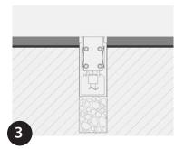
Fill surface gaps with suitable flexible sealing compound. When set remove box cover, make wiring connections and insert MOMO-F. Trim butyl liner flush if used.
