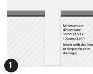
Cast slot from shuttered or solid form to suitable dimensions. If base of slot is not permeable additional drainage may be required.
